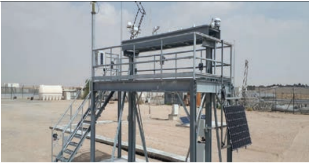
Figure (2): DEWA R&D Radiometric and Aerosols Aeronet Station, Part of NASA Network
