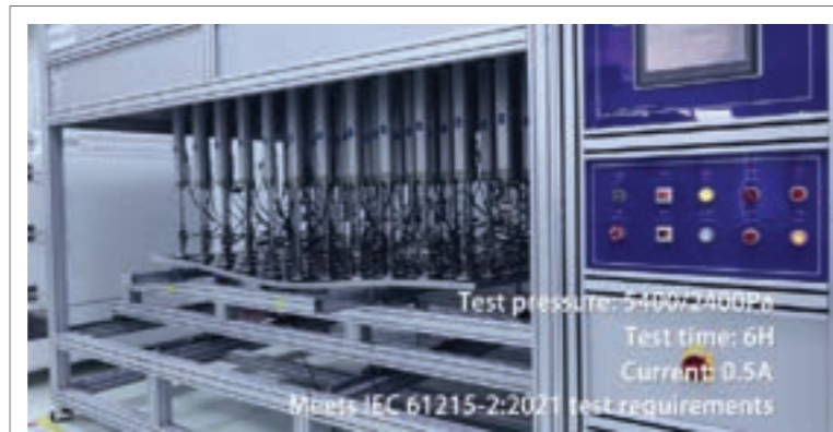
Figure (3): Applying 5400 Pa & 2400 Pa Positive and Negative Pressure to Frontsheet and Backsheet of Panels while Conducting Static Mechanical Load Test Source: DAS Solar Laboratory
